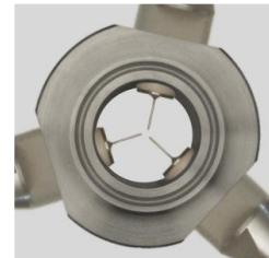
The Keyhole Multi-point probes were mounted at various locations in the process to measure the difference in heating across the radial flow profile.
